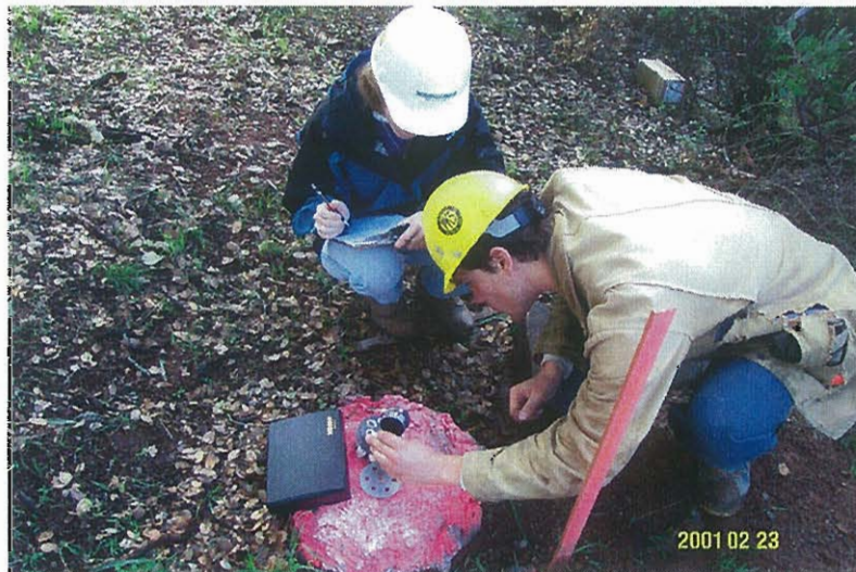
Figure 4-1. Monitoring of MPBX Over a Tunnel
