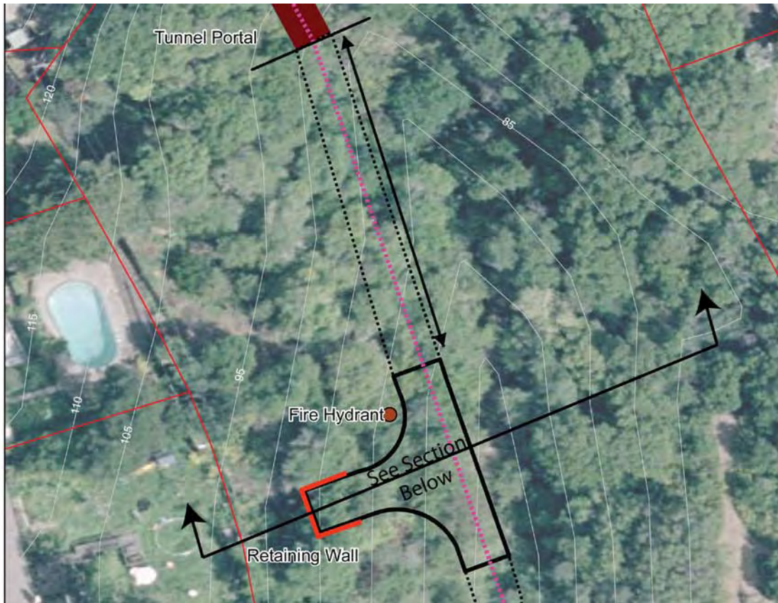
Figure 2-24: South Portal Emergency Vehicle Turnaround Plan
